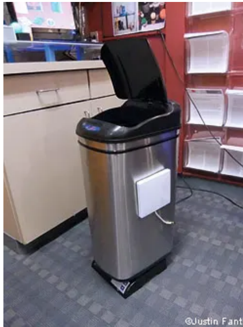
Smart trash can. Part of the AgeLab's 'E-Home project' to redesign living arrangements for older people, the smart trash can uses radio frequency identification (RFID) antennas to tag objects in a kitchen. This allows the bin to sense when items have been used or thrown out – letting distant family members or caregivers look out for unusual eating behaviours
