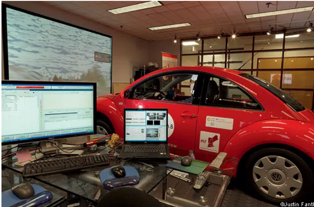
Miss Daisy. Housed in a cherry-red Volkswagen Beetle, Miss Daisy is a driving simulator designed to test the effects of cognitive distraction and medication use on older drivers. The car now sits permanently within the AgeLab, having been winched into the building via a modified elevator shaft
