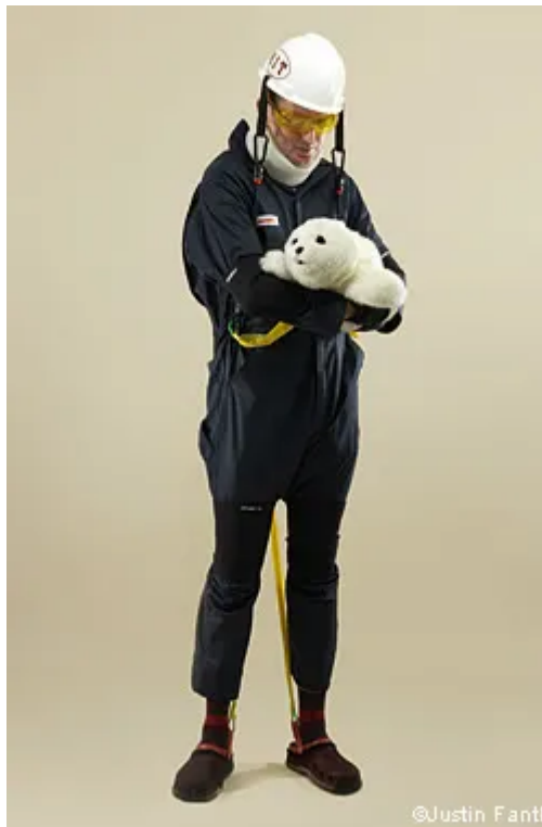
Paro the seal. Paro is an animatronic 'therapeutic' robot baby seal, designed to comfort elderly patients suffering from dementia. Paro responds to touch and sound, waking up and getting sleepy depending on the frequency with which a user interacts with him. Although born in a lab, Paro is now commercially available, with many thousands of units sold in Japan since it was first put on the market in 2003
