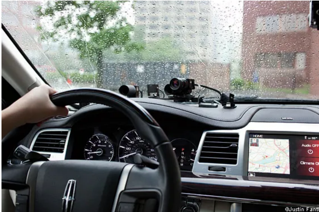
The prototype AwareCar, a souped-up dark red Lincoln MKS, uses on-board eye-tracking cameras to measure the effects of fatigue and distraction on driving ability, while sensors measure heart and breathing rates. The car has helped researchers understand what type of information helps to focus, or distract, elderly drivers on the road
